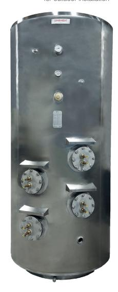
The heat exchanger consists of an outer tin-plated spirally wound high finned tube, and an inner (refrigerant side) copper tube. The double walled structure prevents the possibility of drinking water from mixing with refrigerant oil, meeting DIN standard EN12897 and PD5500.
