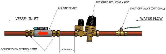
The Air Gap Device can be mounted vertically or horizontally
